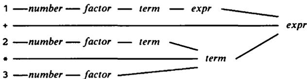
To make an infix evaluator, we need a parser for expressions. With a little effort, the grammar can be used to construct the parser and organize the program as well. A function is written to process each nonterminal in the grammar: the program uses the function `expr` to process *term*'s separated by plus or minus signs, the function `term` to process *factor*'s separated by multiplication or division signs, and the function `factor` to recognize numbers and process parenthesized *expr*'s.
