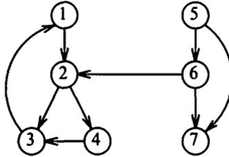
Depth-first search is useful for finding cycles. An edge like (3,1) that goes from a node to a previously visited ancestor is called a *back edge*. Since a back edge identifies a cycle, to find cycles all we need to do is find back edges. The following function will test whether a graph, stored as a successor-list data structure like that in `tsort`, contains a cycle reachable from node:
