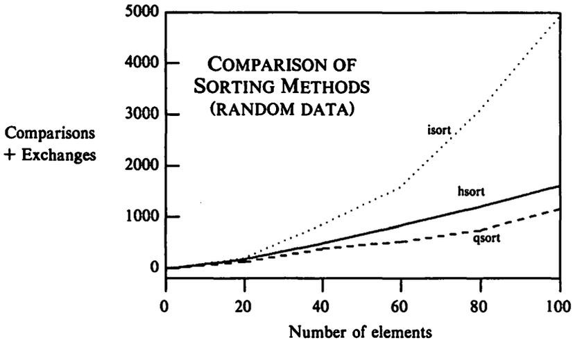
Recall that on random data the performance of *isort* is quadratic while that of *hsort* and *qsort* is  $n \log n$ . The graph clearly shows the importance of good algorithms: as the number of elements increases the difference in performance between the quadratic and the  $n \log n$  programs widens dramatically.
