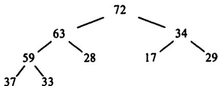
In the next iteration, the first step exchanges elements 72 and 33:
