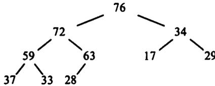
There are two important characteristics of a heap. The first is that if there are  $n$  nodes, then no path from the root to a leaf is longer than  $\log_2 n$ . The second is that the largest element is always at the root (“the top of the heap”).
