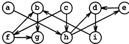
If a graph contains an edge from *x* to *y*, then *x* is called a *predecessor* of *y*, and *y* is a *successor* of *x*. Suppose the constraints come in the form of predecessor-successor pairs where each input line contains *x* and *y* representing an edge from node *x* to node *y*, as in this description of the graph above:
